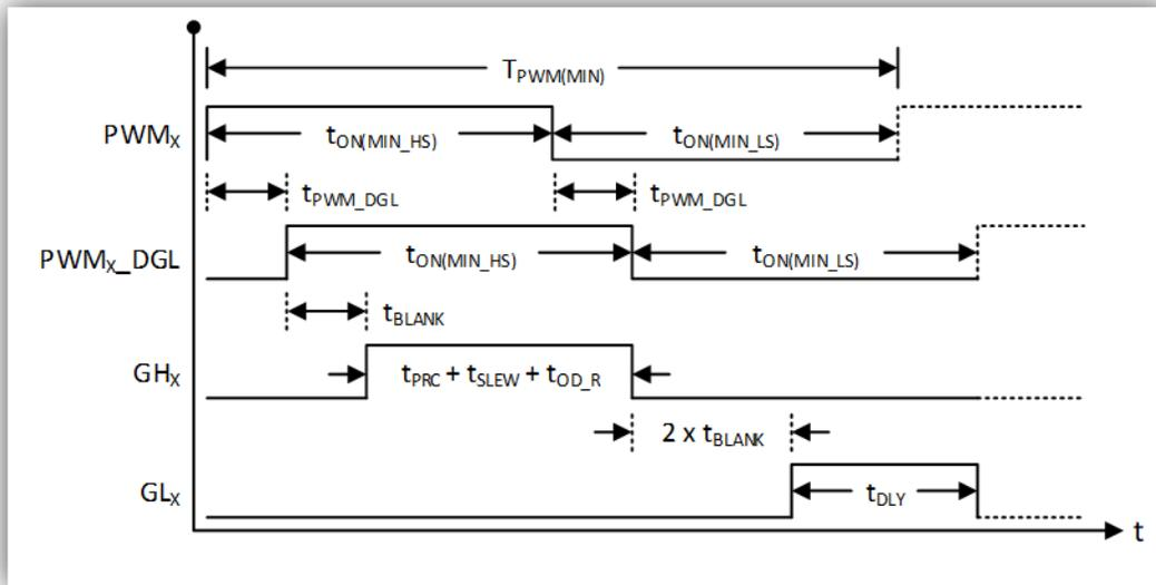
Figure 4. PWM Period Construction
