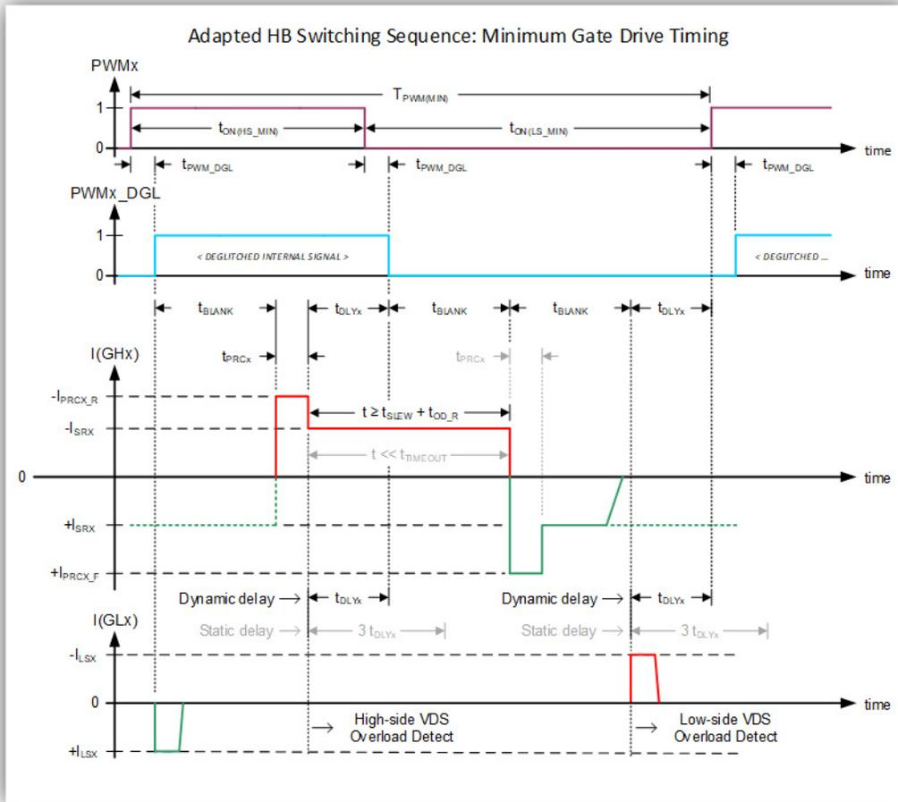
**Figure 3. Adapted Internal Gate Drive Timing**
