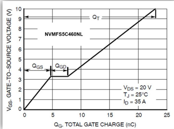
Figure 6. NVMFS5C460NL Datasheet – MOSFET Total Gate Charge Curve
