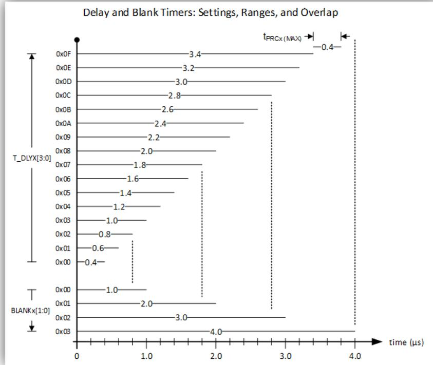
Figure 7. Dynamic VDS Detection Delay and Blanking Time Values – Datasheet Selections
