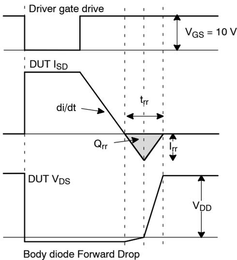
Figure 23. Reverse-Recovery Test Waveforms
