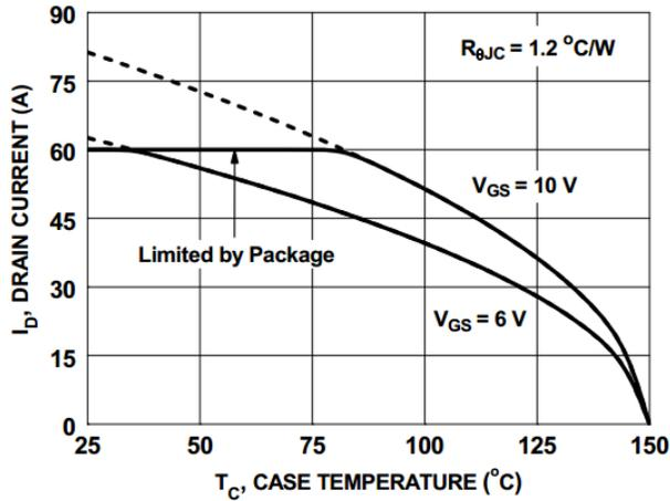
Figure 6. Maximum Continuous Drain Current vs. Case Temperature
