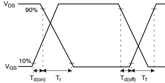
Figure 20. Switching Waveforms
