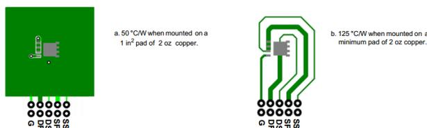
**Figure 5. Mounted PCB Information for Thermal Resistance**
