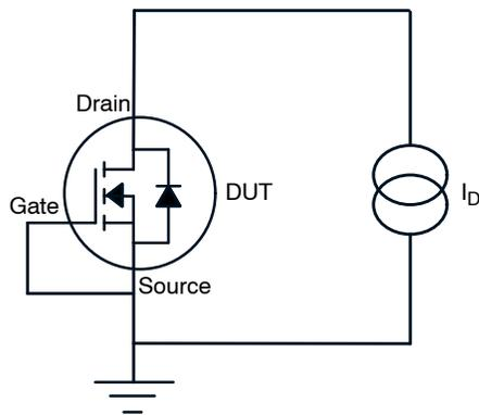
Figure 1. Drain-to-Source Breakdown Voltage Test Circuit
