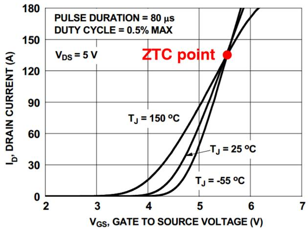
Figure 9. Transfer Characteristics
